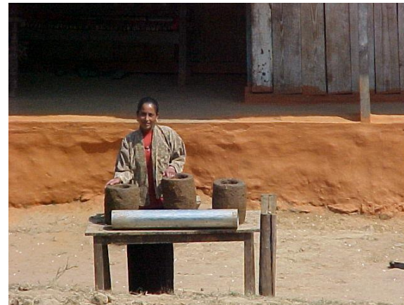
Materials Used – Mud Klin (like traditional oven) with metal sheet chimney pipe and iron grate
